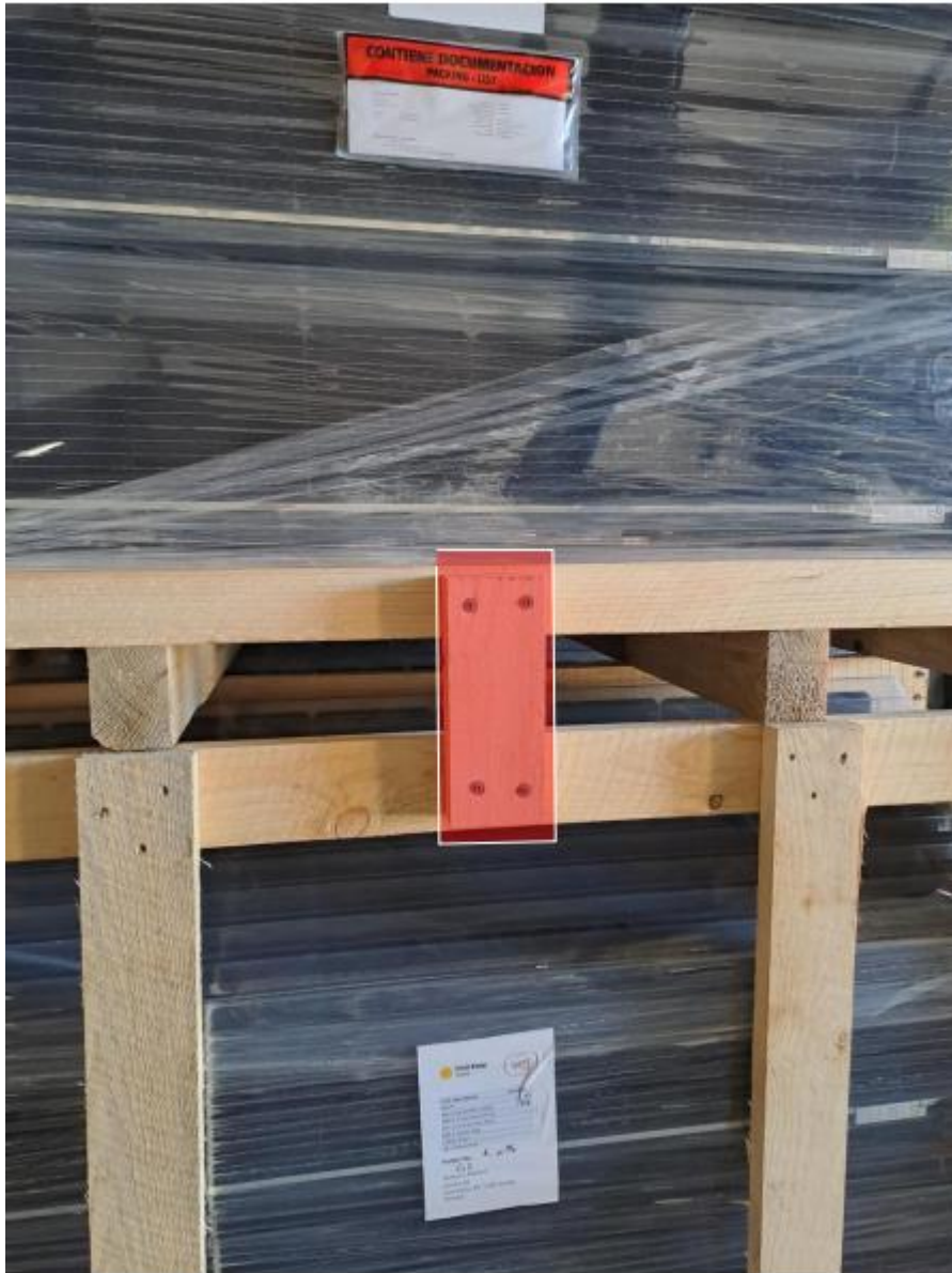
Figure 4: Screws connecting the upper and lower pallets
